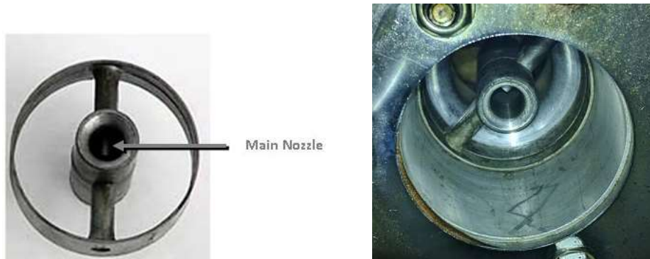
Figure 41. Auxiliary Venturi (part and installed)
