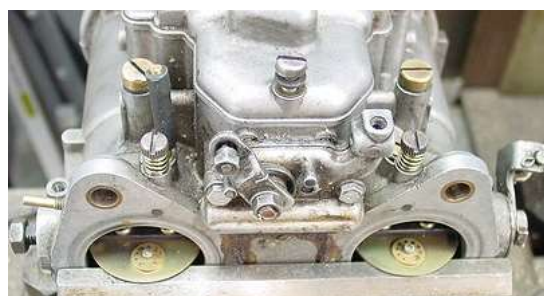
Figure 48. Modified Throttle Plates with Adjustable Sized Holes.
