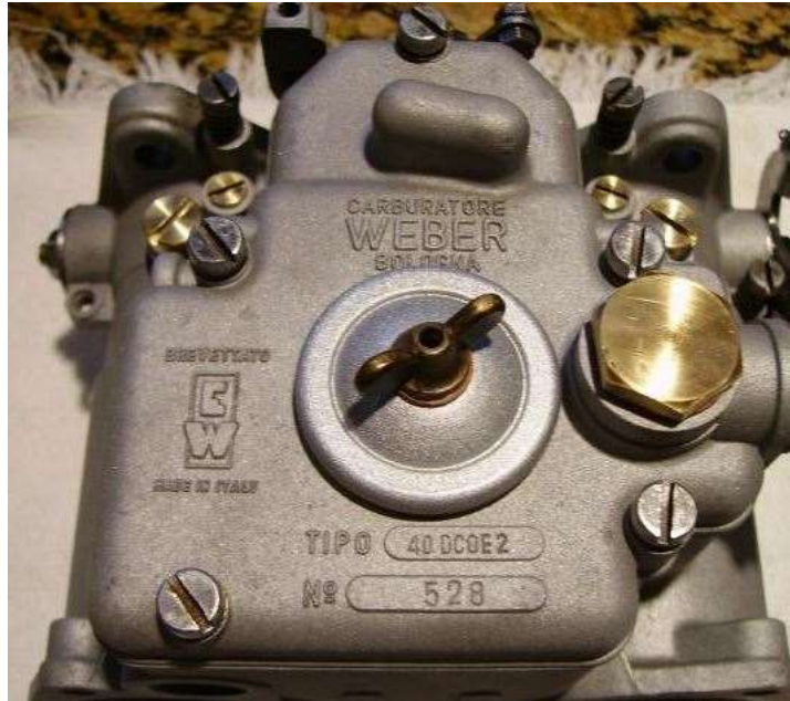
Figure 36. 40DCOE2 Carburetor (Type/TIPO is 2 and stamped on top cover)
