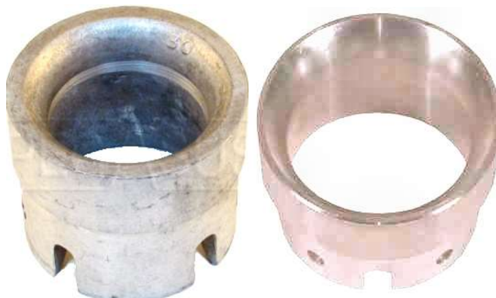
Figure 38. A thick-walled 30mm Venturi and a thin-walled 36mm Venturi
