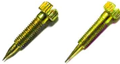
Figure 49. Idle Enrichment Screws (older, wider taper on left, newer, narrower taper on right)
