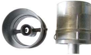
Figure 42. 40DCOE Auxiliary Venturi is just one part. (The 45DCOE Aux. Venturi is two parts)
