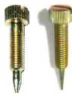
Figure 12. DCOE Idle Enrichment Screws (Two common types shown above with different tapers however at least six existed as part numbers end with: 1,3,11,23,56,58)
