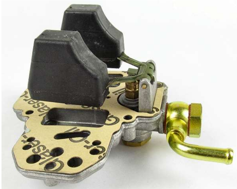
Figure 55. DCOE Lid (upside down) Showing Float, Needle Valve, Gasket and Fuel Inlet
